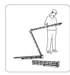
Set frame to desired height then extend legs accordingly and fasten with black knob
